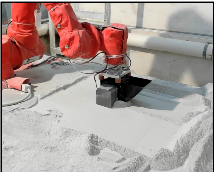
Figure 1: MEERCAT Plate Compaction
